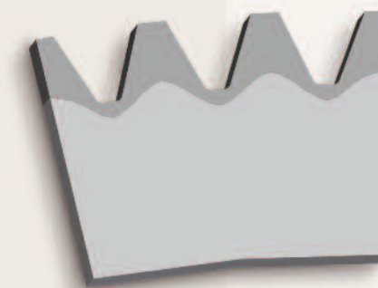
induction hardening of entire gear
