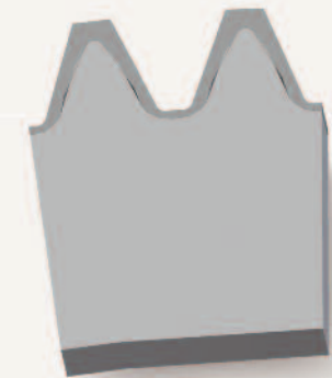
induction hardening of tooth side and bottom
